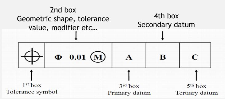
The third, fourth and fifth boxes provide information about datum. If it is necessary to specify more than one tolerance characteristic for a feature, the tolerance specifications are given in the tolerance frames one under the other.
