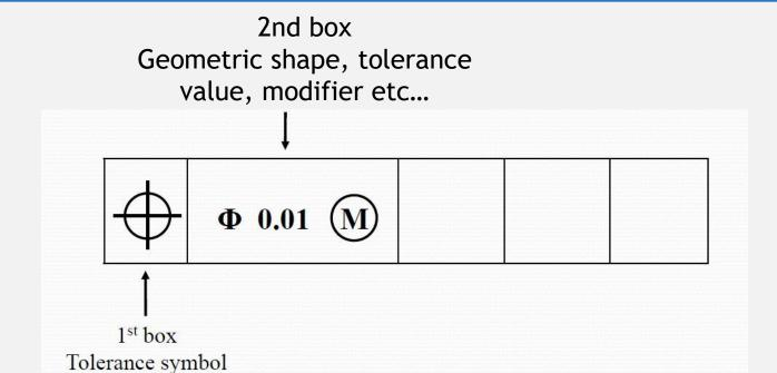
The next or second from left box gives the information about the nature of geometric shape, its tolerance value and modifiers that describe the tolerance conditions.
