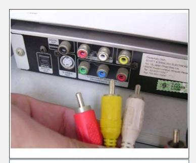
Initial problem: RCA cables was wrongly inserted into the jacks
