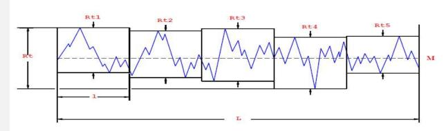
Maximum Height of the Profile, Rt, the vertical distance between the highest and lowest points of the profile within the evaluation length.
